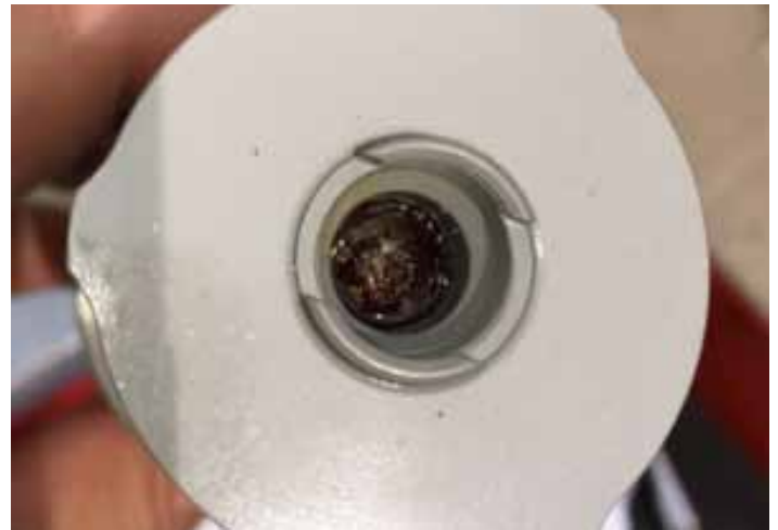
A corroded check valve (ABOVE) can lead to contaminated fuel. (LEFT) Contaminated fuel is shown after being drained from an aircraft tank.
