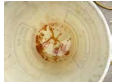
A corroded check valve (ABOVE) can lead to contaminated fuel. (LEFT) Contaminated fuel is shown after being drained from an aircraft tank.
