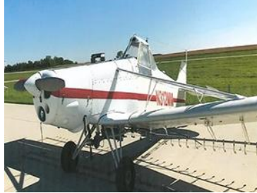
1976 PIPER PAWNEE N312MM 6,067 A/F TT, Lycoming O-540- 132C5, 9,335.48 TTE, 540.0 TSMOS, Salto Lite Star 3 Boom, CP-3 Nozzle
