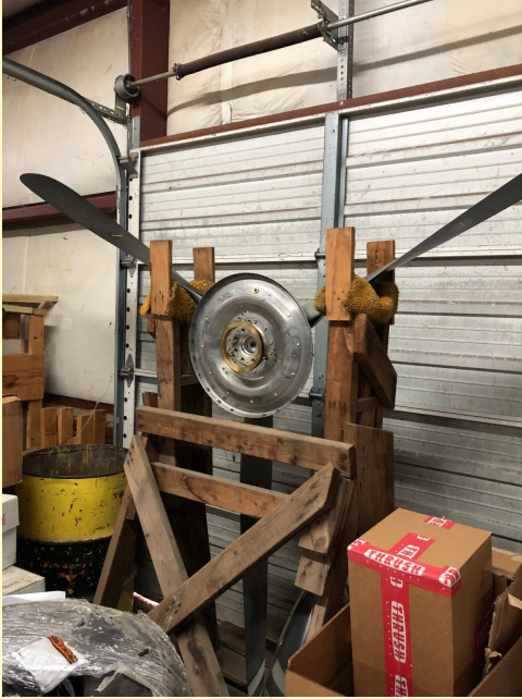
+4 Three-Blade Prop HCB3TN3D/T10282N Only 5.15 hours ferry time
