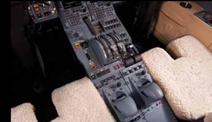
Honeywell's EPIC system lets you switch displayed information on the MFD easily via dual cursor control devices on the center pedestal.
